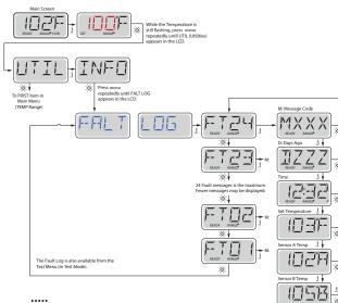
Waiting several seconds inside the Fault Log Menu will allow the screen to return to normal operation.
