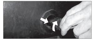
Step 4: Remove drain cap.
