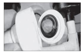
Step 4: Replace filter screen and re-tighten fitting.
