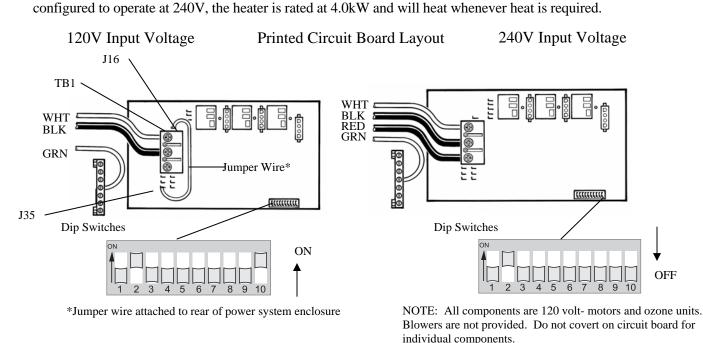
When configuring the output voltages on the FreeFlow SUV System, remember to also consider the amperage of
