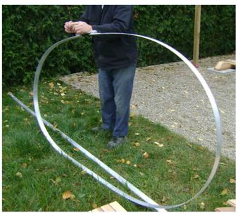
Assemble two of the bands so they can be slipped easily on over the ends of the barrel.
