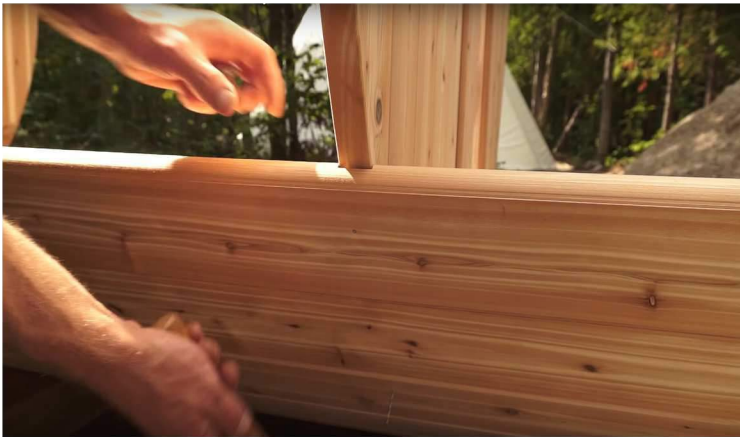
17. On bottom staves, use provided 2 1/2" nails to hold staves in place. ( If needed) nailing every other stave.
