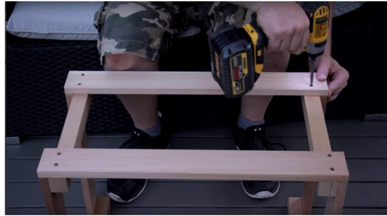
HG-2. Assemble remaining front support to the 2 ends in the same manner as previous step.
