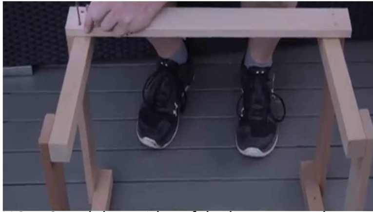
HG-1. Stand the 2 sides of the heater guard on edge with predrilled holes on the bottom. Screw front guard support to either side using 2 1/2" screws. (2 screws per side)
