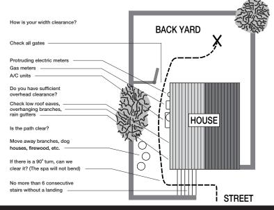
It may be necessary to remove a gate, part of a fence, or other movable obstructions in order to roll the spa to its installation site. About ten percent of the time, a crane is the only way to install the spa by lifting it to its final destination.
