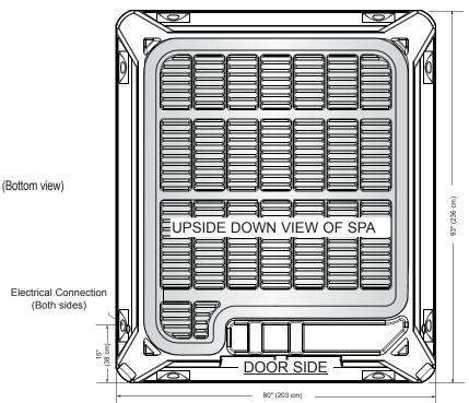
**NOTE: WATKINS WELLNESS** recommends that the **SOVEREIGN** be installed on a minimum 4" (10 cm) thick reinforced concrete pad or a deck that is able to withstand more than 110 lbs/ft² (535 kg/m²).
