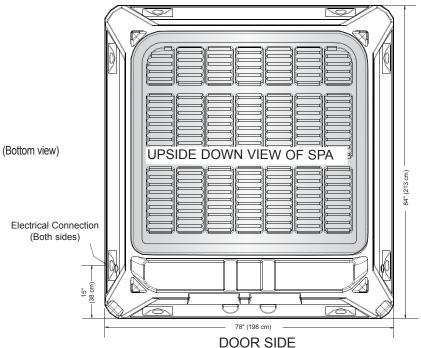
**NOTE: WATKINS WELLNESS** recommends that the **PRODIGY** be installed on a minimum 4" (10 cm) thick reinforced concrete pad or a deck that is able to withstand more than 110 lbs/ft² (535 kg/m²).
