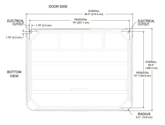
**NOTE: WATKINS WELLNESS** recommends that the STRIDE be installed on a minimum 4" (10.2 cm) thick reinforced concrete pad or structurally sound deck able to support the "dead weight" found in the spa specification chart.
