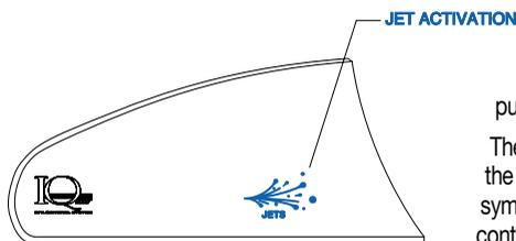
The **CLEAN** button, provided as a convenient timer for water maintenance, activates the jet pump for a ten minute period. The CLEAN indicator will turn on and the JET symbol on the display will illuminate to indicate the jet pump is engaged. Next you may add properly measured spa water chemicals into the filter compartment. The jet pump and clean indicator will automatically shut off after 10 minutes.
