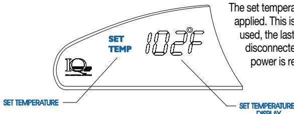
The set temperature of the spa water will automatically be 102°F the first time that power is applied. This is the setting programmed at the factory. After the spa has been set up and used, the last temperature value set by the user will be stored in memory. If power is disconnected from the spa, it will automatically revert to the last set temperature when power is reappplied.
