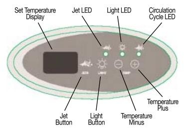
C. TEMPERATURE CONTROLS: The set temperature range is from 50°F to 104°F (10°C to 40°C). Higher temperatures can be reached by using one of three codes: U1, U2 and U3. These are progressively warmer, with U3 the highest at approximately 106°F. (The temperature of any setting may rise slightly depending on the current use and condition of your spa, and outside temperature.)
